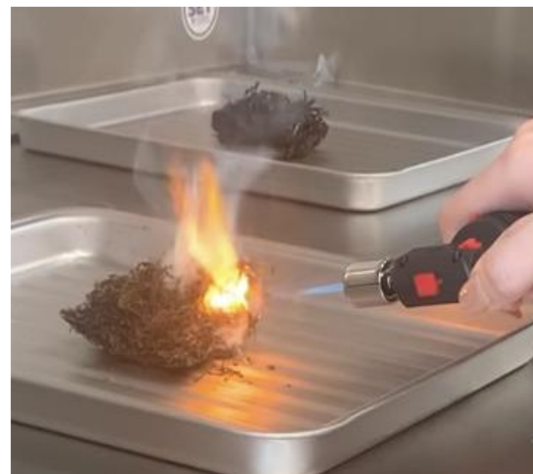
Image of burn testing being conducted on a Sargassum sample
