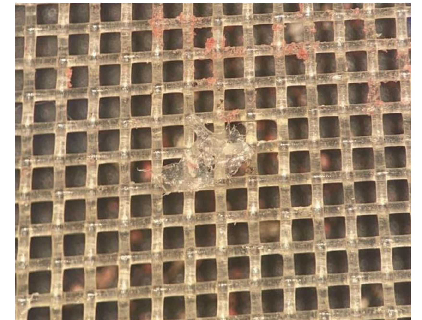
Film microplastic recovered from 0.33 mm sieve
