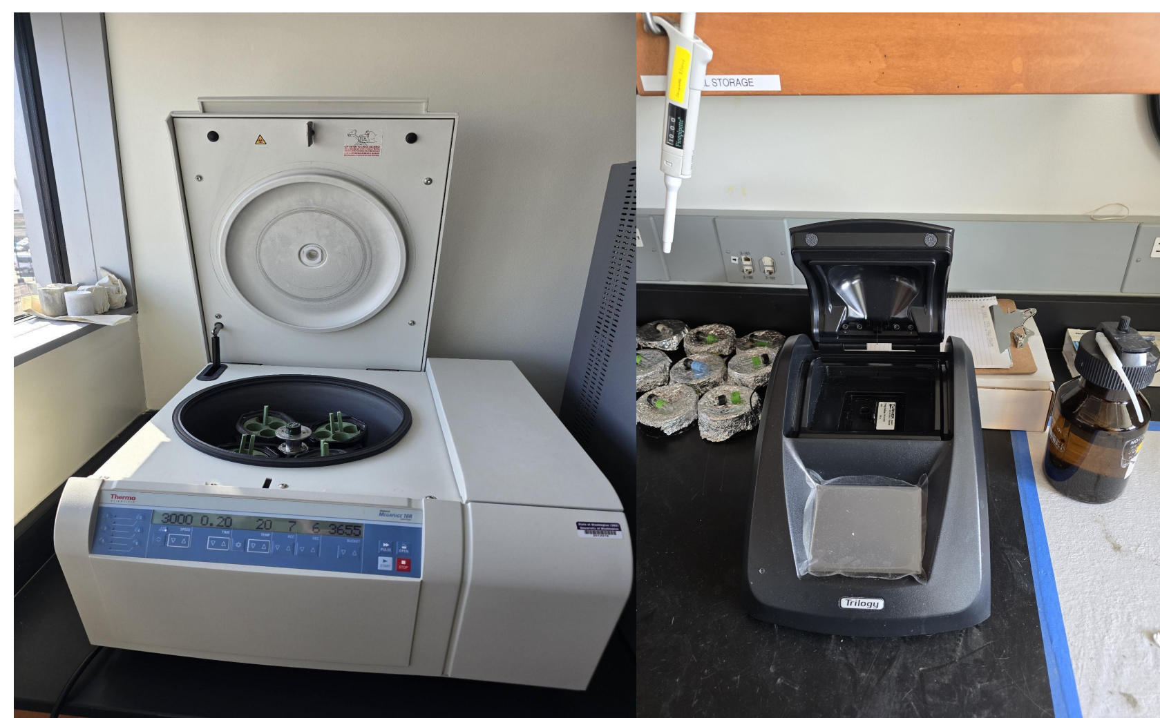
Figure 1: Images of Centrifuge and Fluorometer used for separation and fluorescent analysis of chlorophyll-a concentration.
