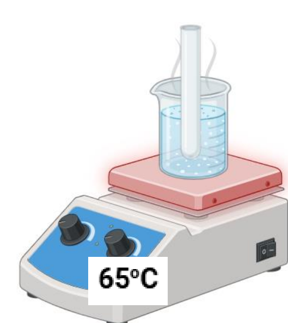
Figure 4. Chemical Synthesis Process. Quinazolinone, solvent, and base are sequentially combined, followed by the addition of methyl bromoacetate. The reaction mixture is heated to 65 °C for 90 minutes. Conditions such as solvent and base identity were varied in different experiments.
